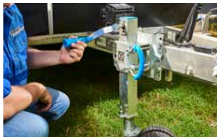
Lower the jockey wheel to take the weight of the trailer
