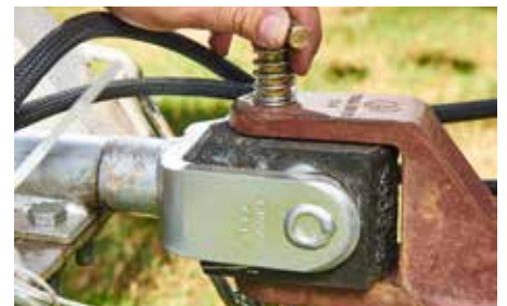
Ensure that the pin in your Treg hitch has no pressure on it
