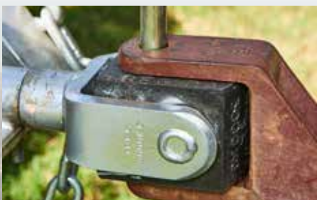
Now remove your Treg hitch pin completely
