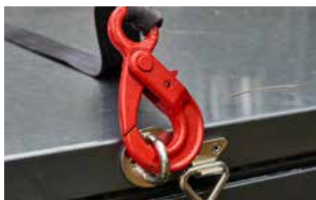
Attach hooks to the anchor points
