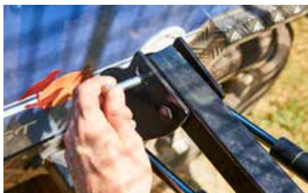
Remove the locking bolts
