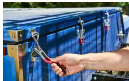
Release the over-centre catches
