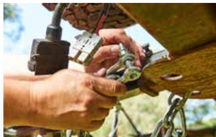
Don't forget the safety chains
