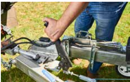
Set the handbrake
