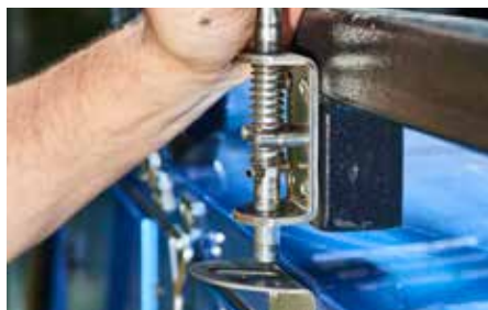
Unlock the locking pin
