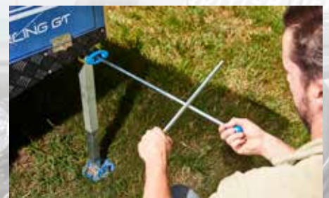
Lower all legs into position & Use your winch tool to level the trailer
