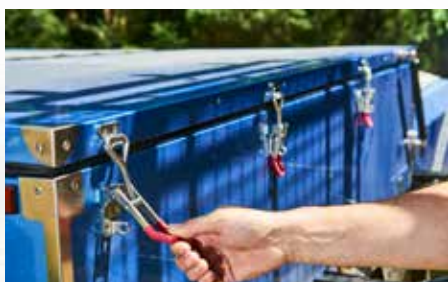
Release the over-centre catches
